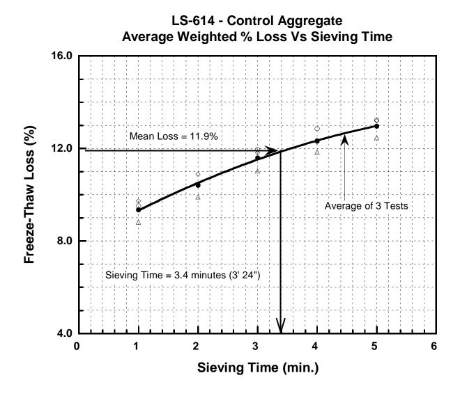
**Figure A1 -** Plot of Average Weighted Freeze-Thaw Loss of Control Aggregate Vs Time (The time of 3 min 23 sec is established for quantitative sieving of samples when prepared, tested, and evaluated using sieve set A and shaker X).
