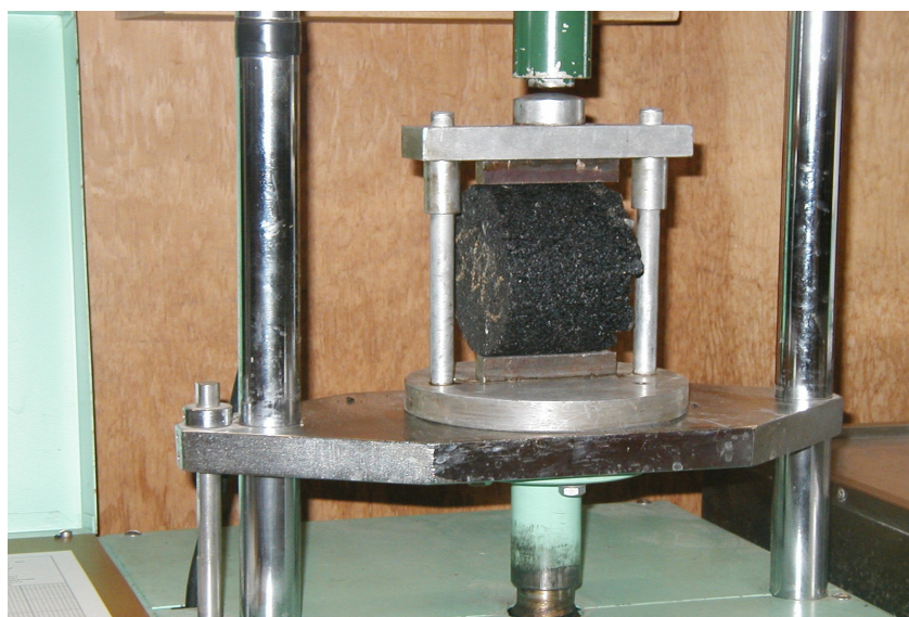
Figure 1 Humboldt Modified Lotman Breaking Head with Guide Rods and Loading Strips
