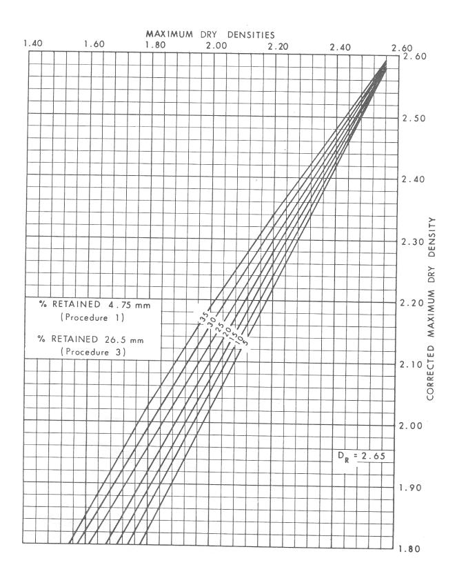
Figure 2 Plus 4.75 mm Correction Table for Dry Densities
