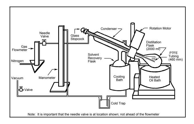
Figure 4 Rotavapor Apparatus And Recovery System (Option B)
