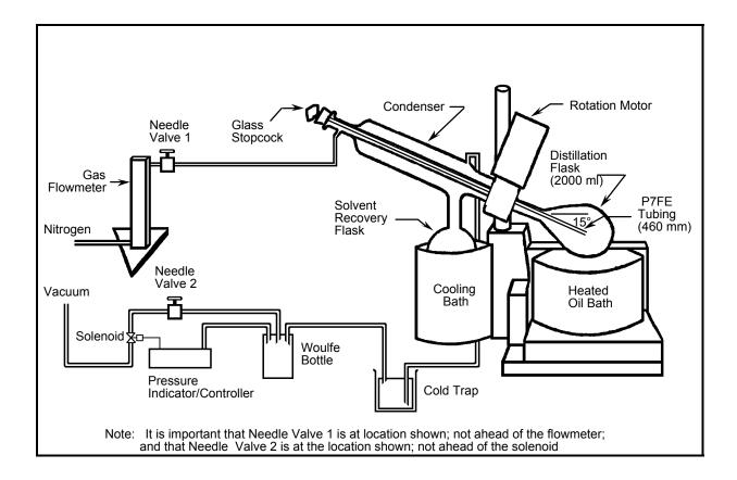
Figure 5 Rotavapor Apparatus And Recovery System (Option C)
