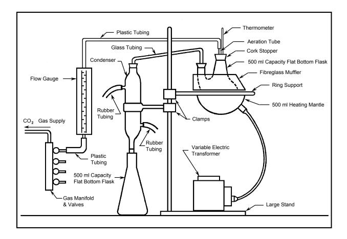
Figure 2 Abson Secondary Distillation System
