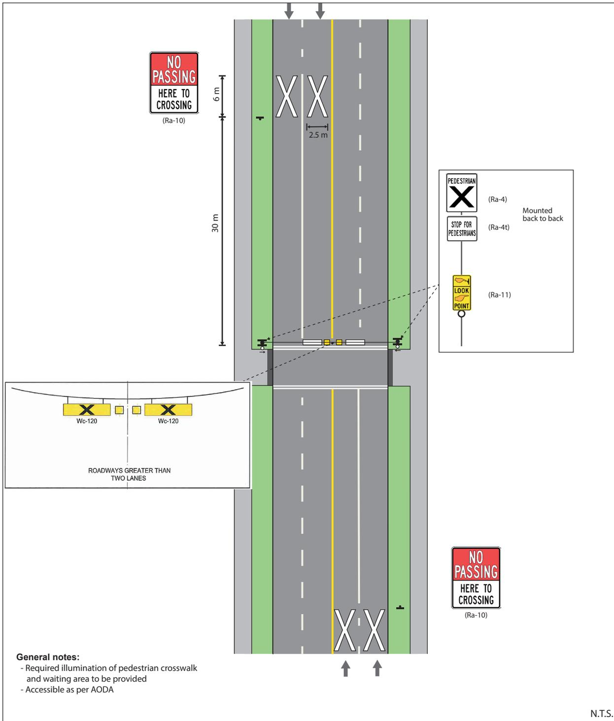
Figure 21: Pedestrian Crossover Type A – Mid-block (4-lane, 2-way)
