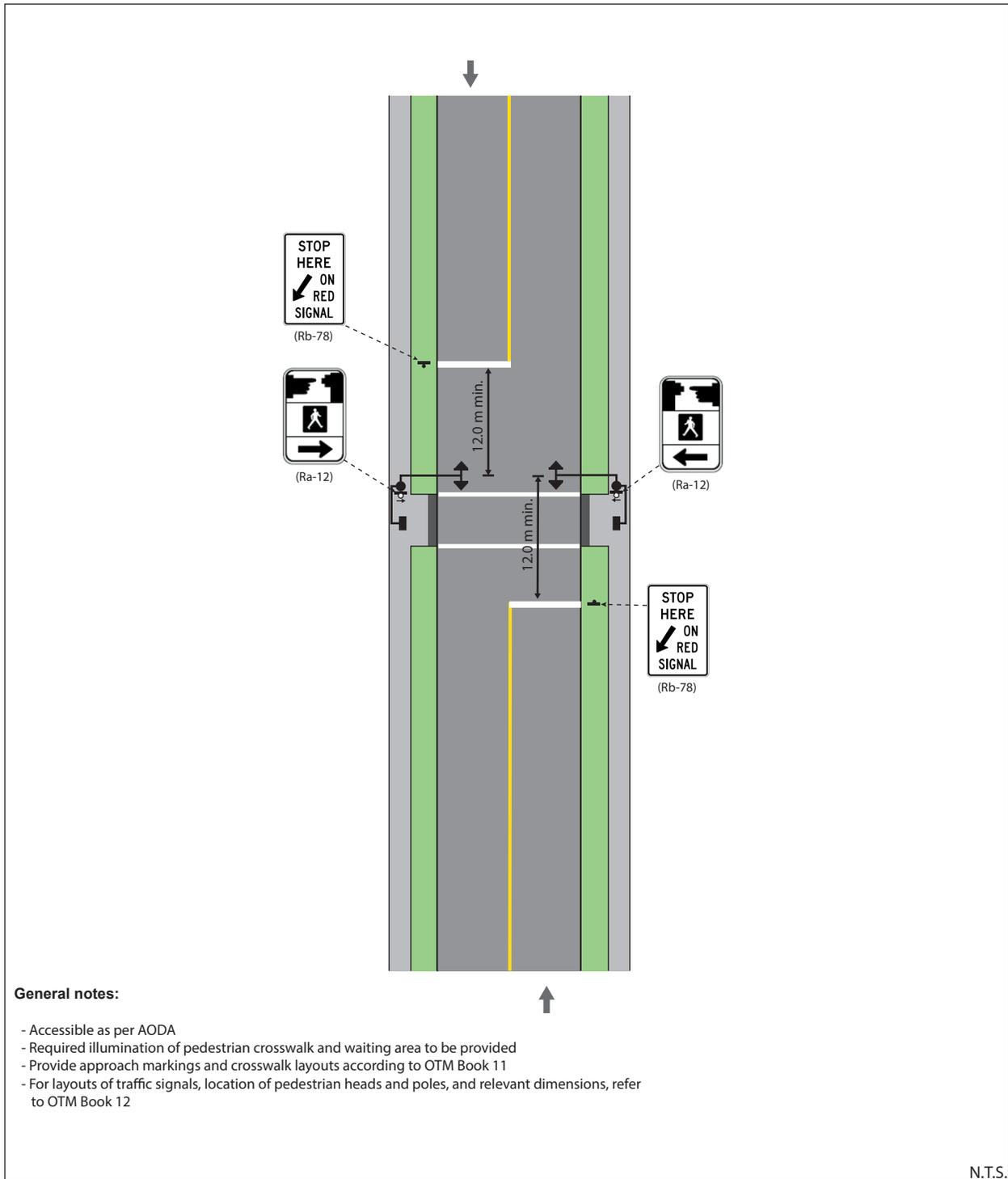
**Figure 18: Mid-block Pedestrian Signal Pedestrian Crossing Treatment (2-lane, 2-way)**
