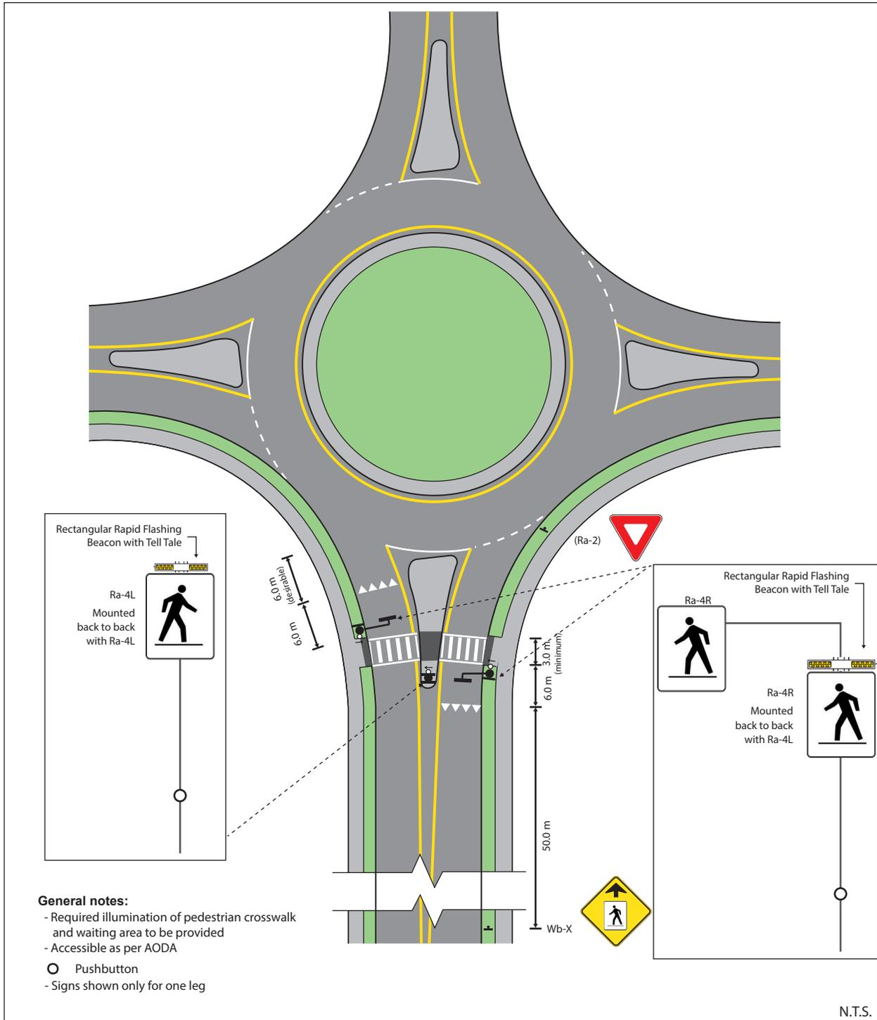
Figure 29: Pedestrian Crossover Type B – Single-Lane Roundabout
