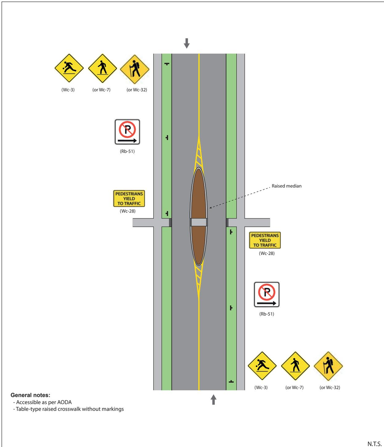
Figure 53: Typical Uncontrolled Pedestrian Crossing with Raised Median
