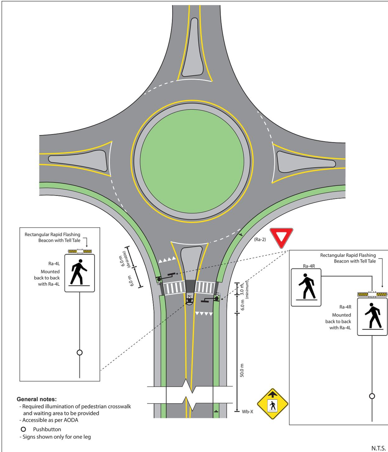
**Figure 38: Pedestrian Crossover Type C – Single-Lane Roundabout**
