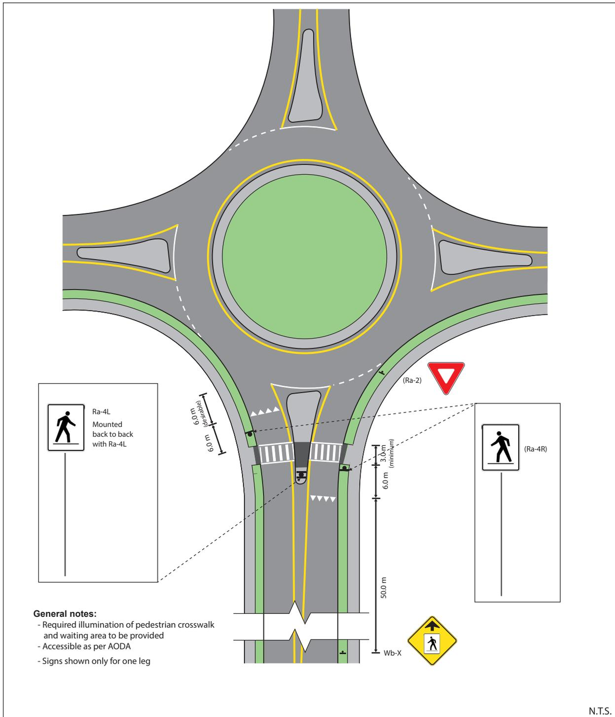
Figure 46: Pedestrian Crossover Type D – Single-Lane Roundabout
