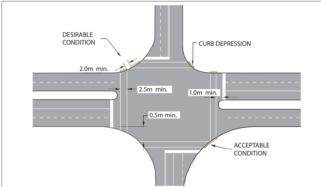
**Figure 8: Typical Crosswalk Design with Standard Crosswalk Markings**
