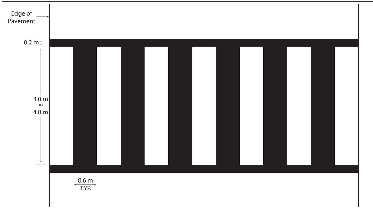
**Figure 13: Pavement Markings for Ladder Crosswalk**
