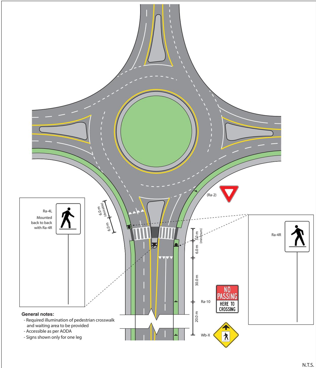
Figure 47: Pedestrian Crossover Type D – Double-Lane Roundabout
