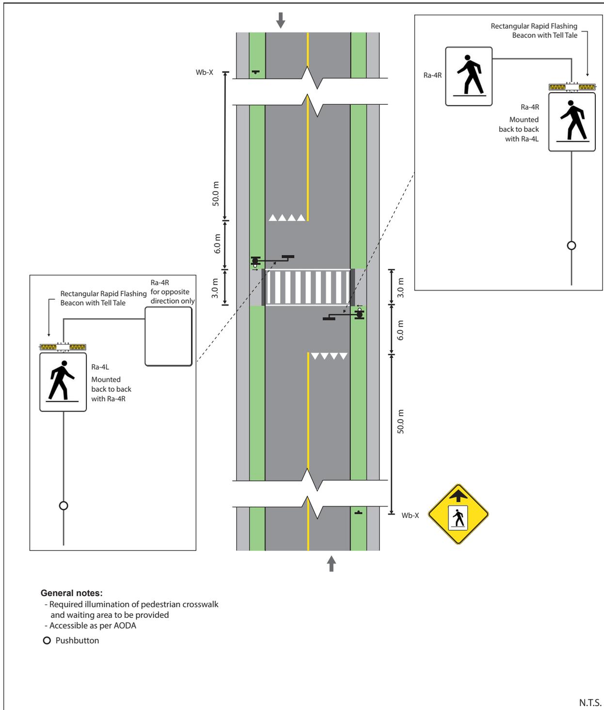
Figure 22: Pedestrian Crossover Type B – Mid-block (2-lane, 2-way)
