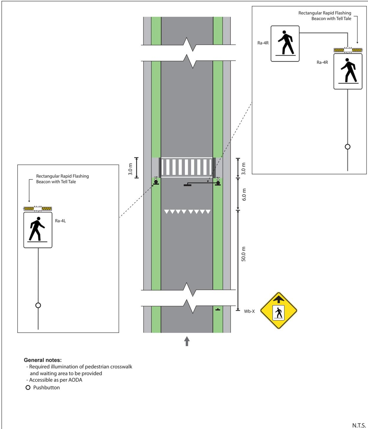
Figure 25: Pedestrian Crossover Type B – Mid-block (1-lane, 1-way)
