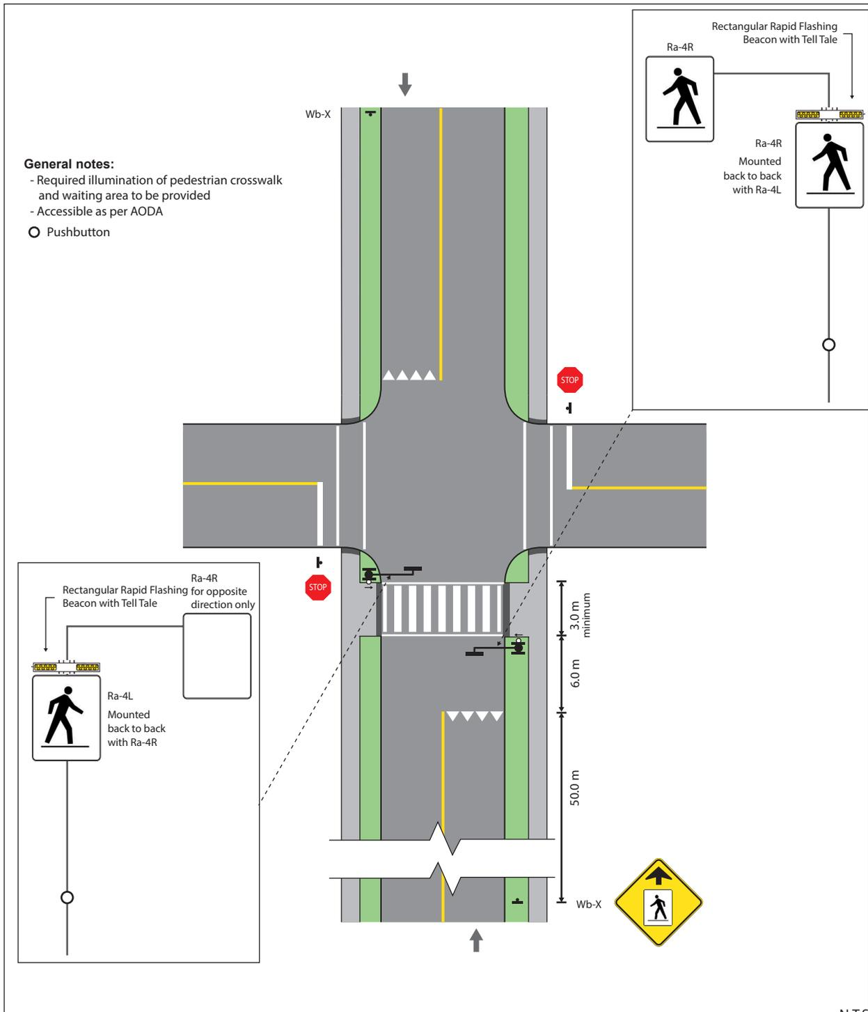
Figure 28: Pedestrian Crossover Type B – Intersection (2-way)
