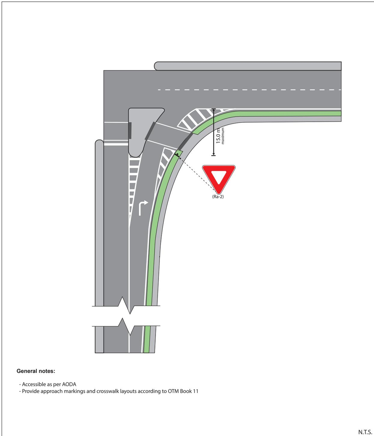
**Figure 50: Yield Controlled Intersections as Pedestrian Crossing Treatment**
