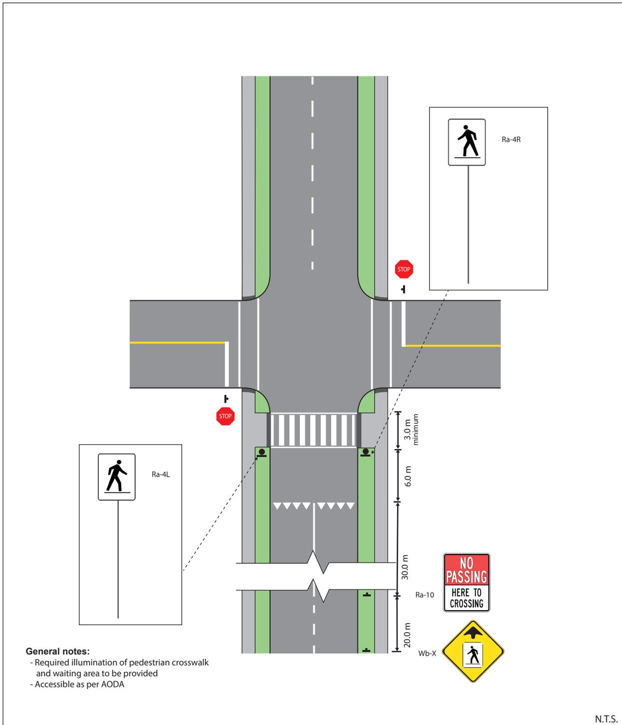
Figure 44: Pedestrian Crossover Type D – Intersection (1-way)
