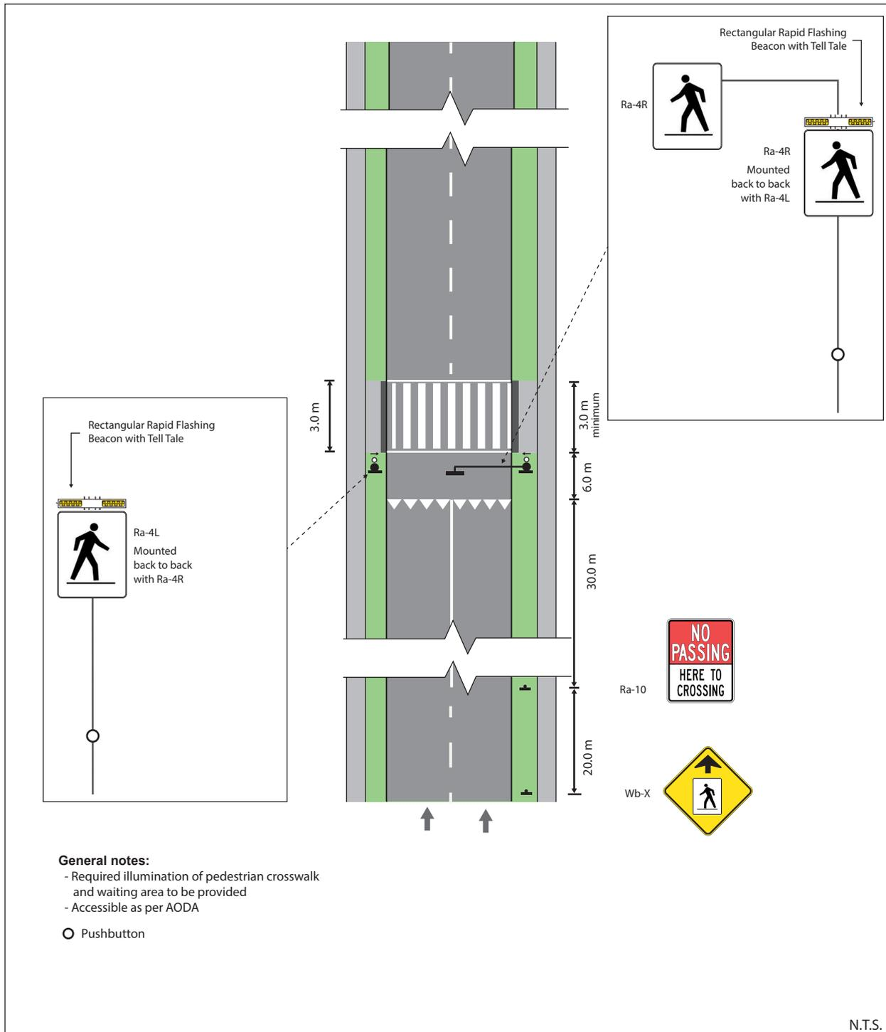
Figure 26: Pedestrian Crossover Type B – Mid-block (2-lane, 1-way)
