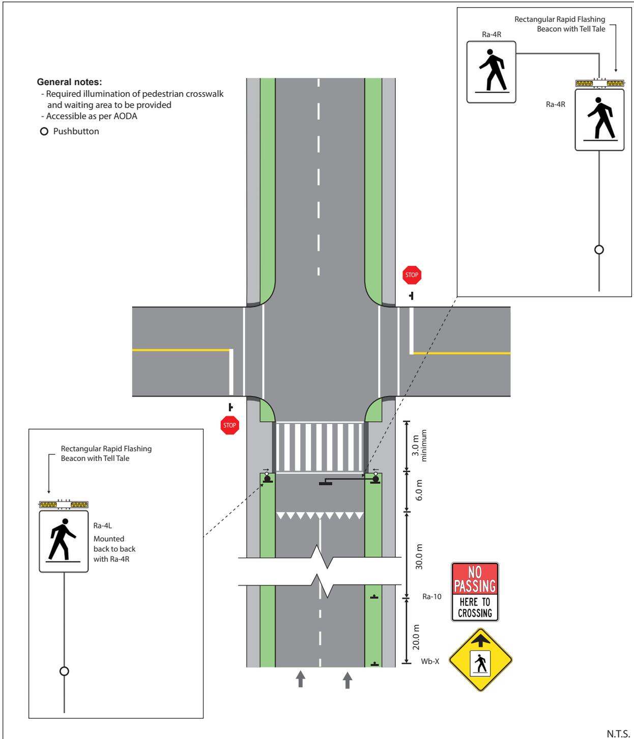
Figure 27: Pedestrian Crossover Type B – Intersection (1 –way)
