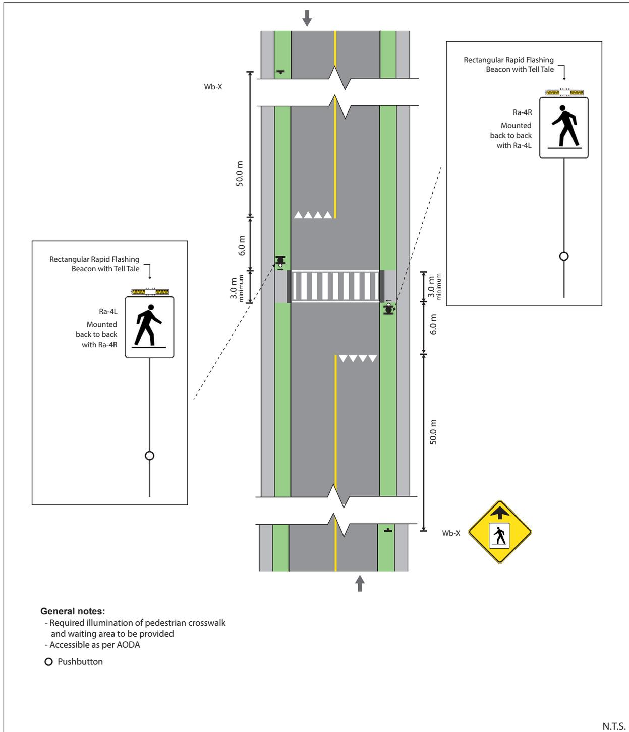
Figure 31: Pedestrian Crossover Type C – Mid-block (2-lane, 2-way)
