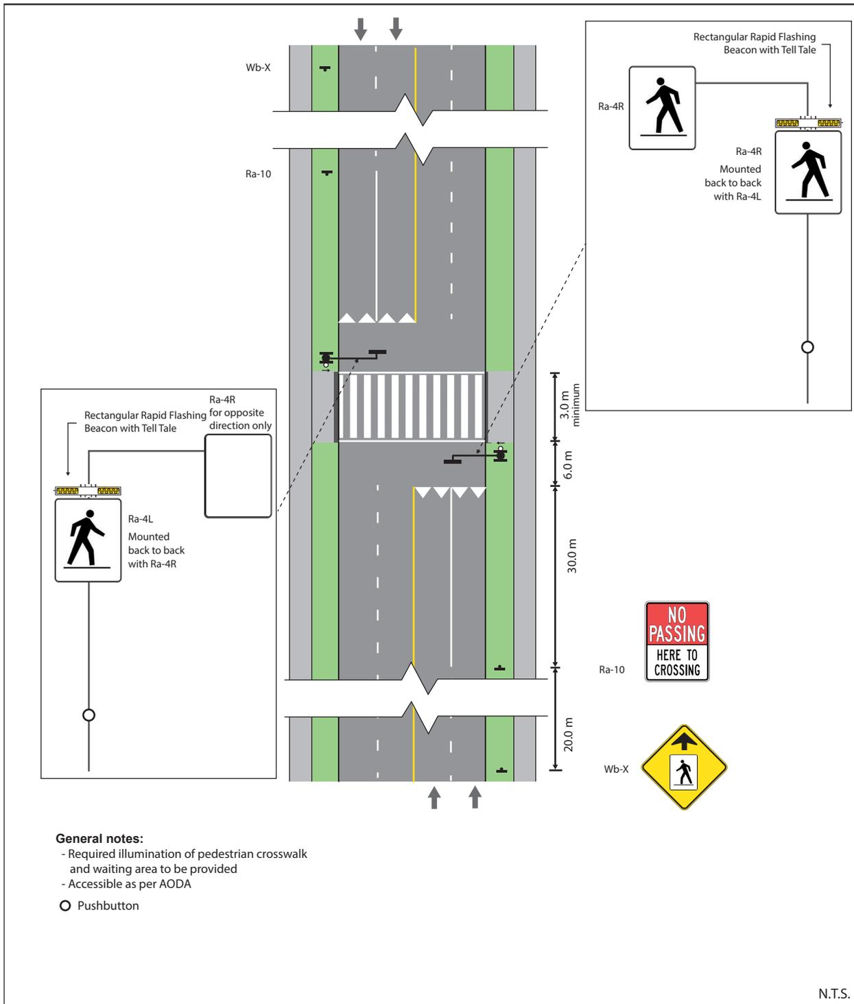
Figure 24: Pedestrian Crossover Type B – Mid-block (4-lane, 2-way)
