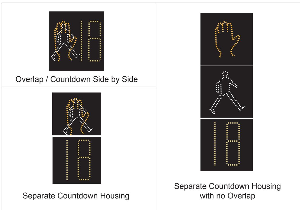
**Figure 9: Pedestrian Countdown Timers Display Configuration**
