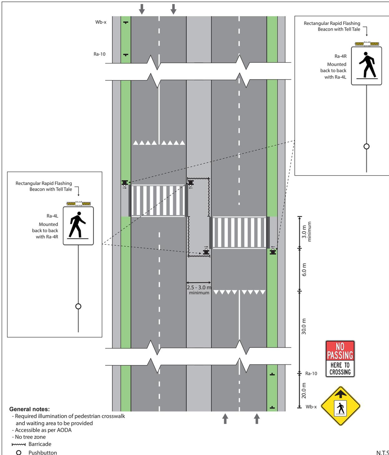
Figure 33: Pedestrian Crossover Type C – Mid-block (4-lane, 2-way with raised refuge)
