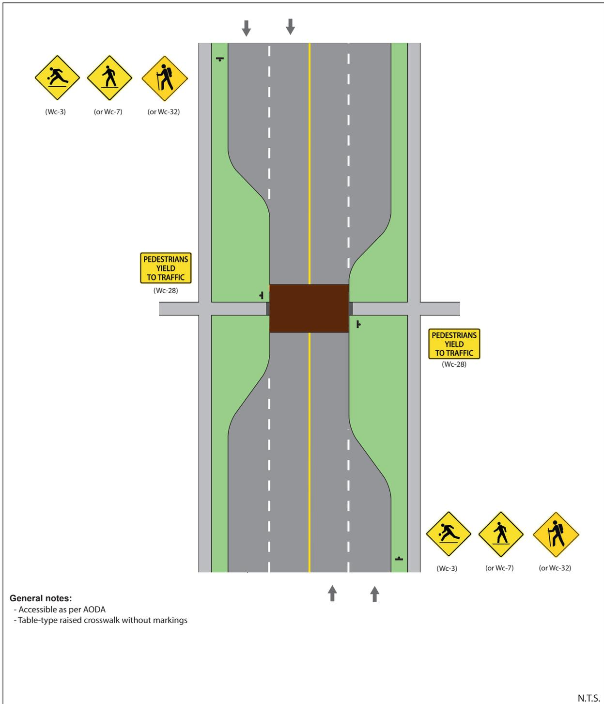
**Figure 54: Typical Uncontrolled Pedestrian Crossing with Raised Crosswalk**
