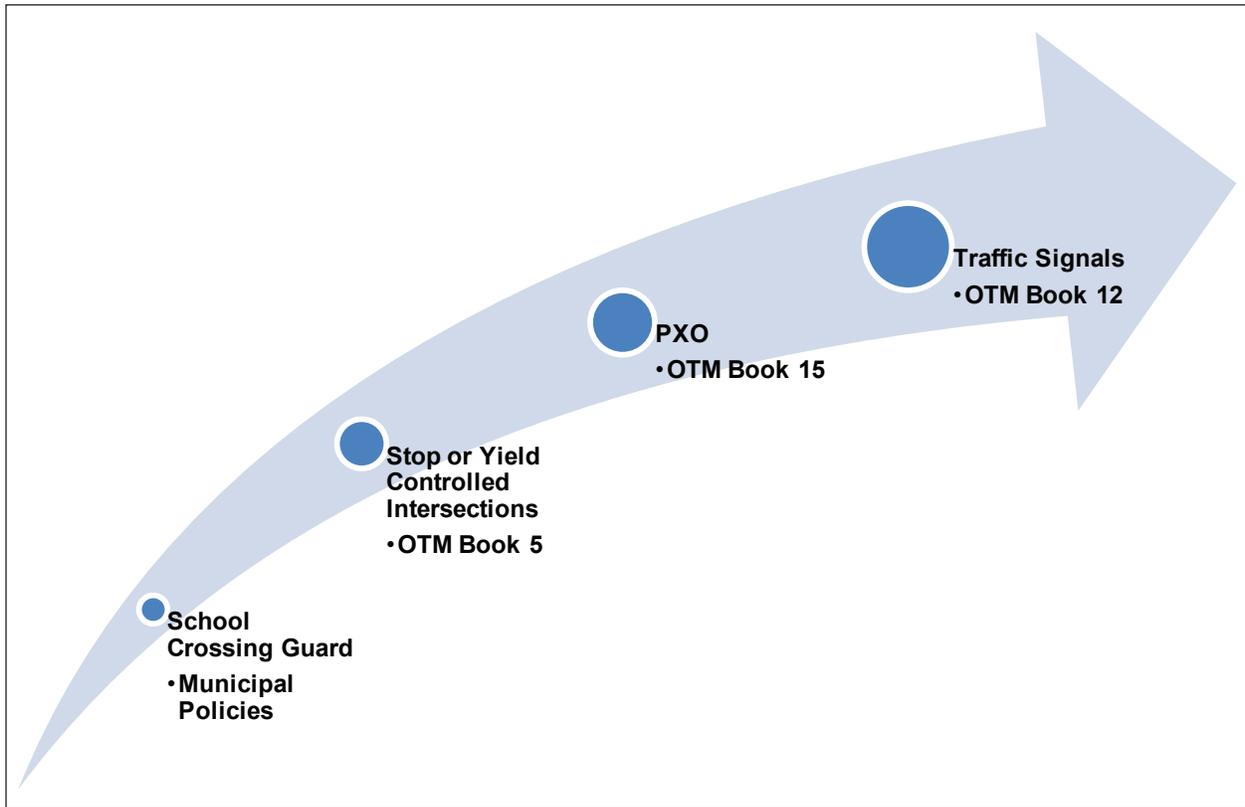
**Figure 2: Hierarchy of Controlled Crossing Treatment Systems and Current Policies and Guidelines**
