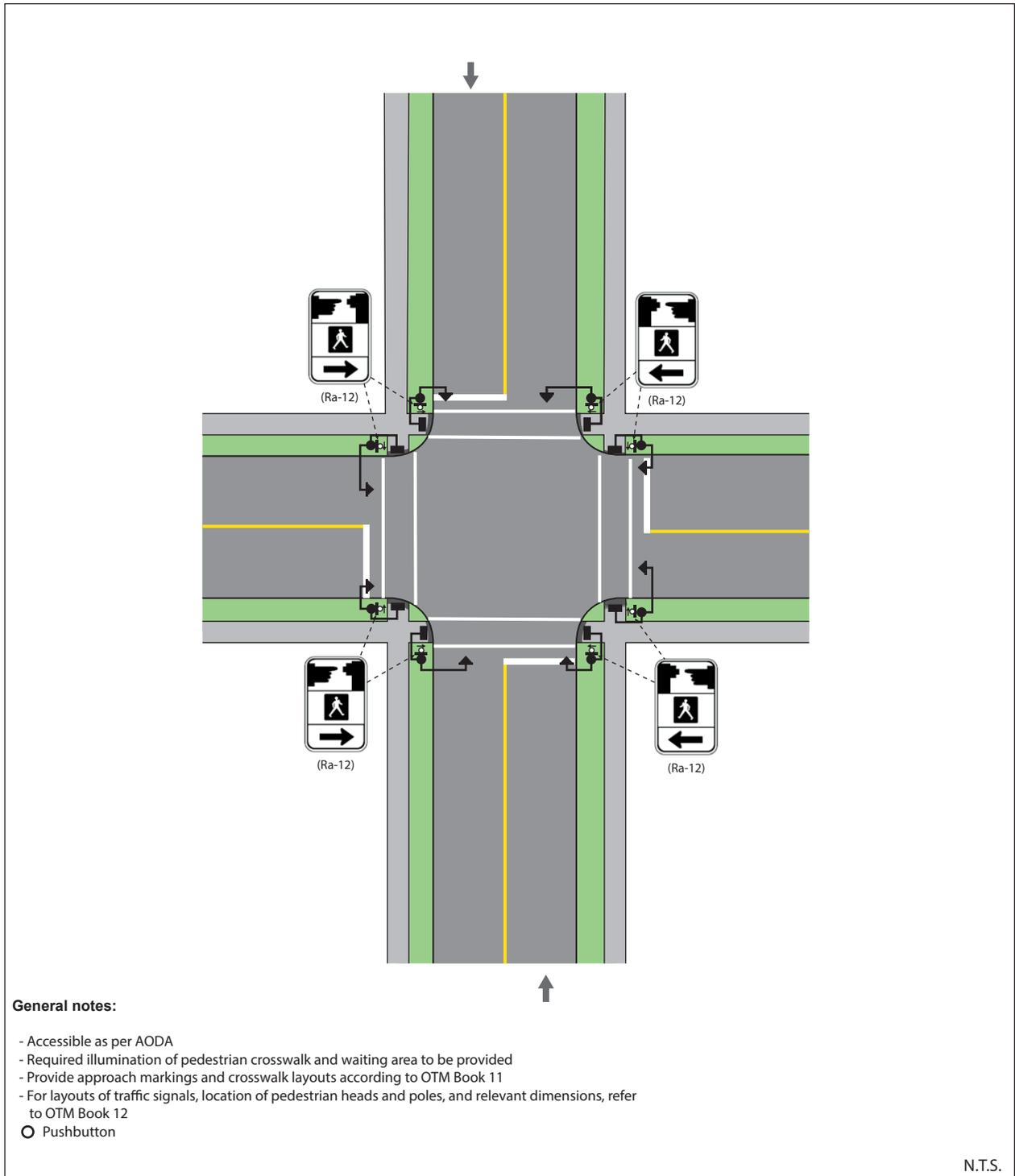
**Figure 14: Pedestrian Treatment at Full Traffic Signal (2-lane, 2-way)**
