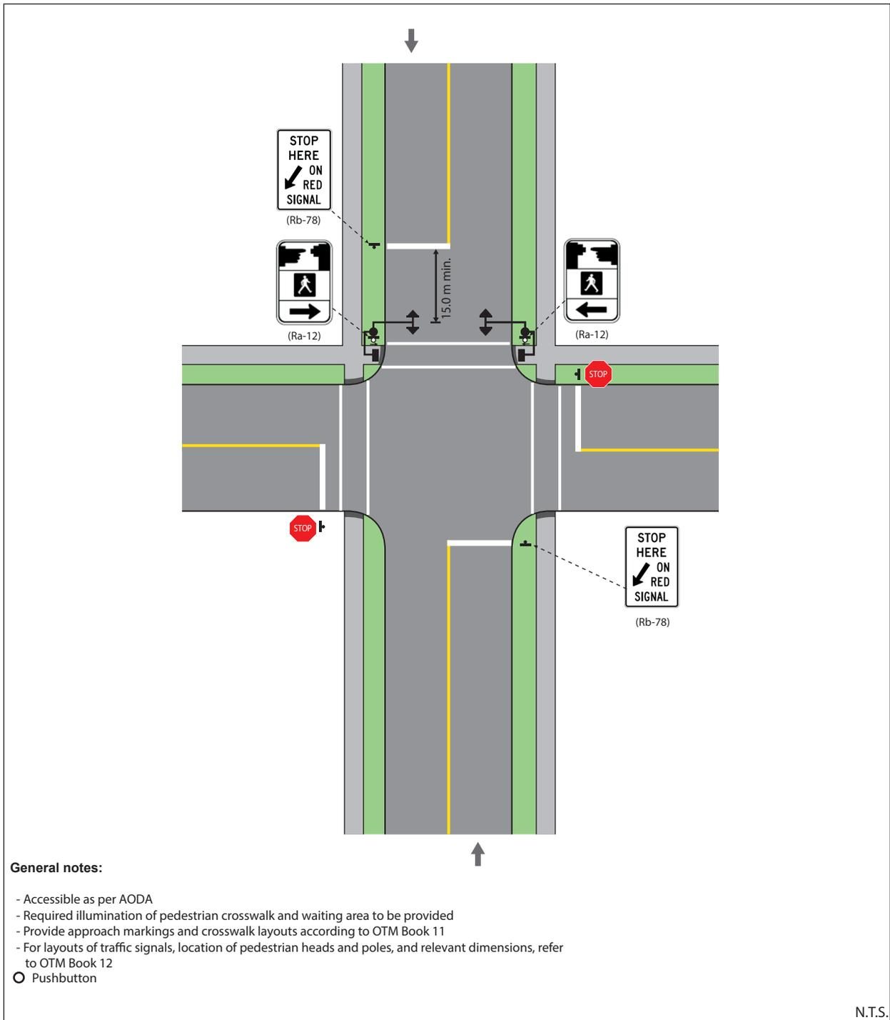
**Figure 16: Intersection Pedestrian Signal Pedestrian Crossing Treatment (2-lane, 2-way)**
