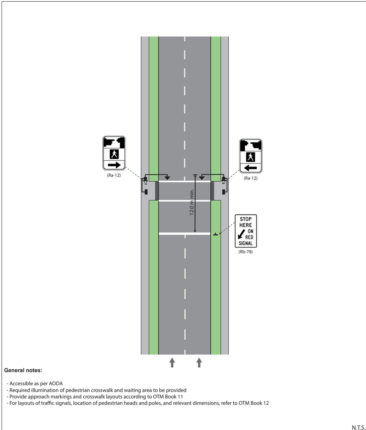
**Figure 19: Mid-block Pedestrian Signal Pedestrian Crossing Treatment (2-lane, 1-way)**
