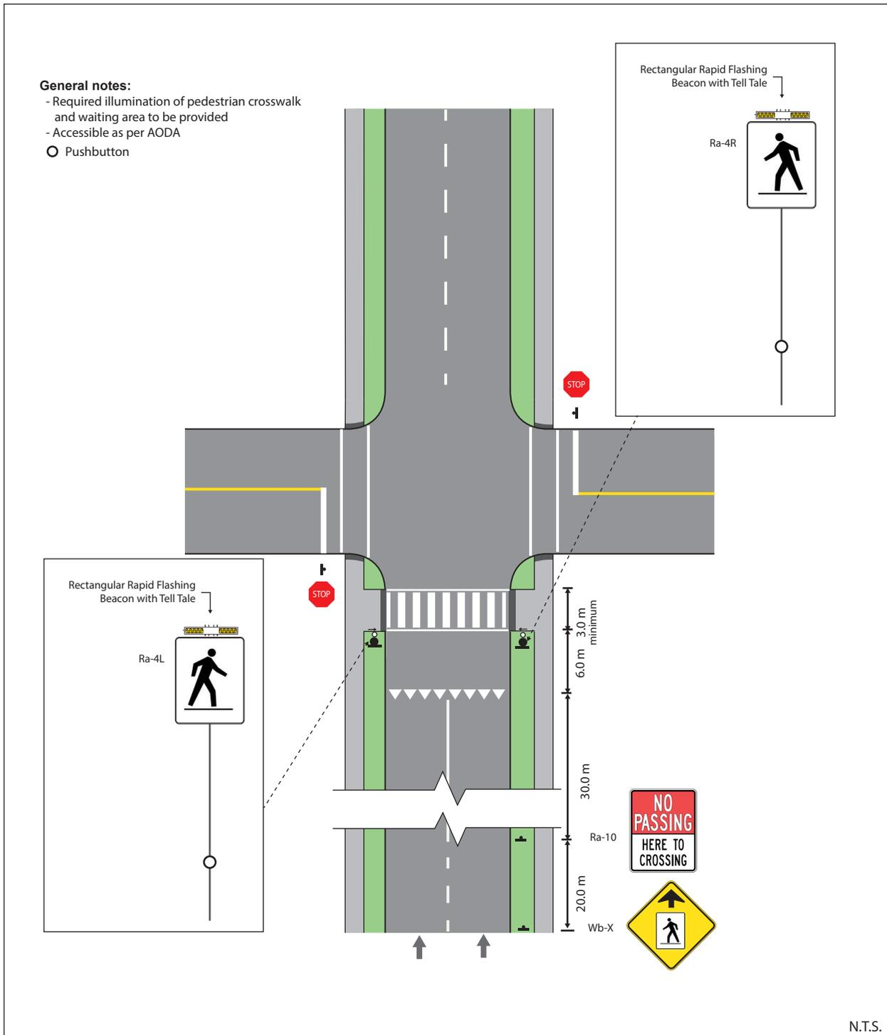
Figure 36: Pedestrian Crossover Type C – Intersection (1-way)
