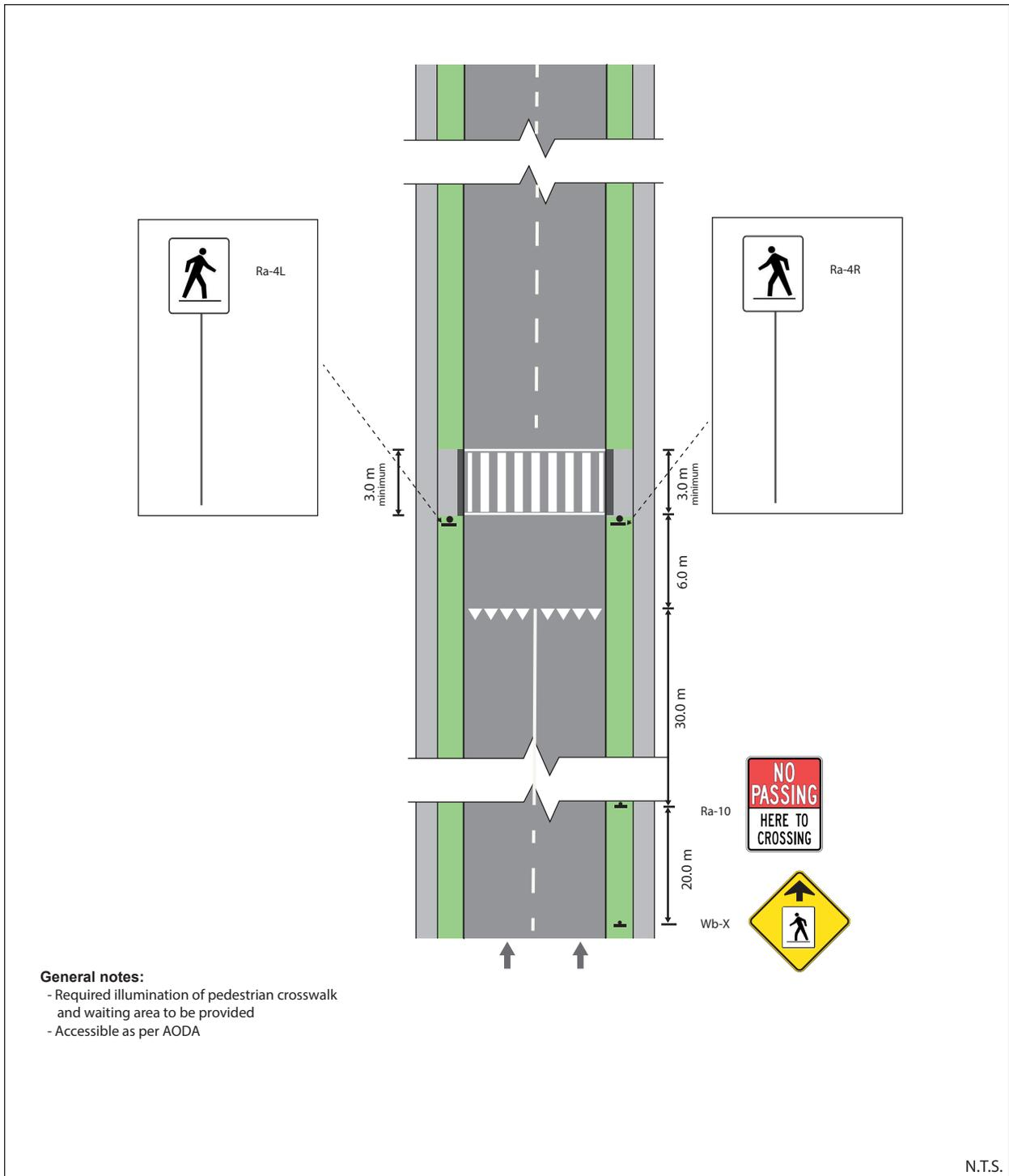
Figure 43: Pedestrian Crossover Type D – Mid-block (2-lane, 1-way)
