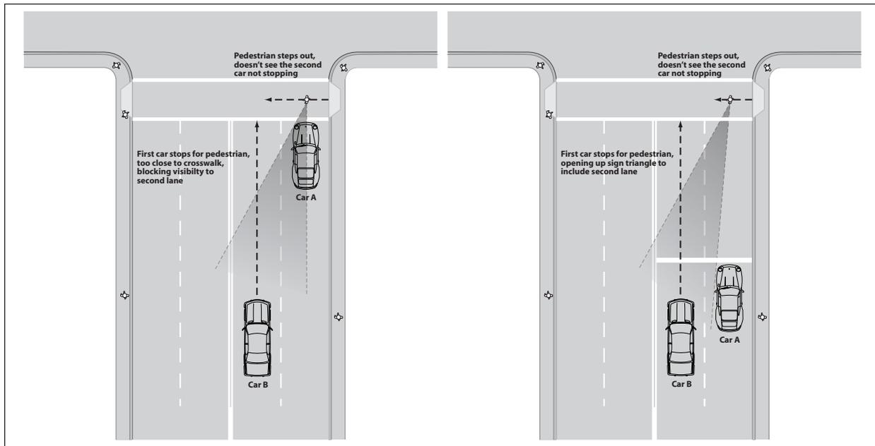
Figure 11: Pedestrian Visibility with Advanced Stop Bar
