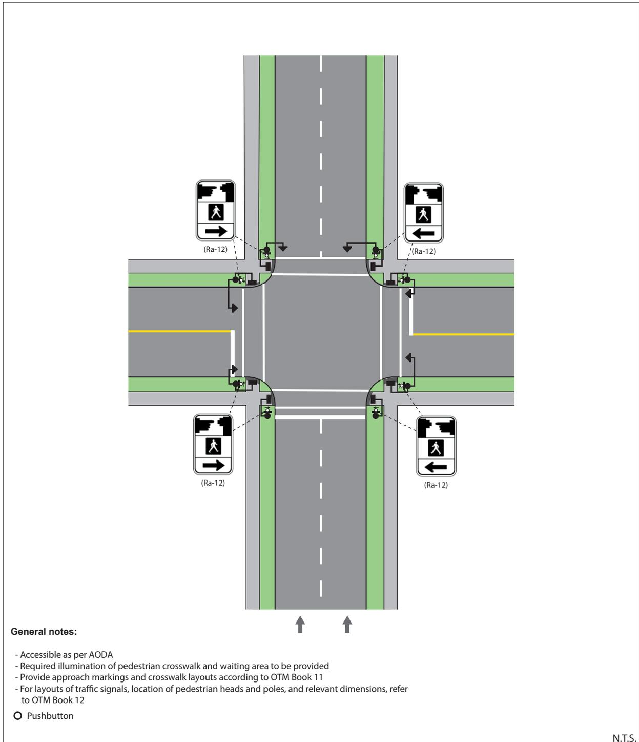
**Figure 15: Pedestrian Treatment at Full Traffic Signal (2-lane, 1-way)**
