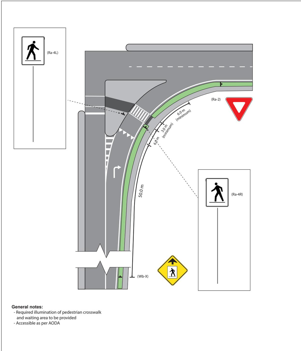
Figure 48: Pedestrian Crossover Type D – Right-turn Channel
