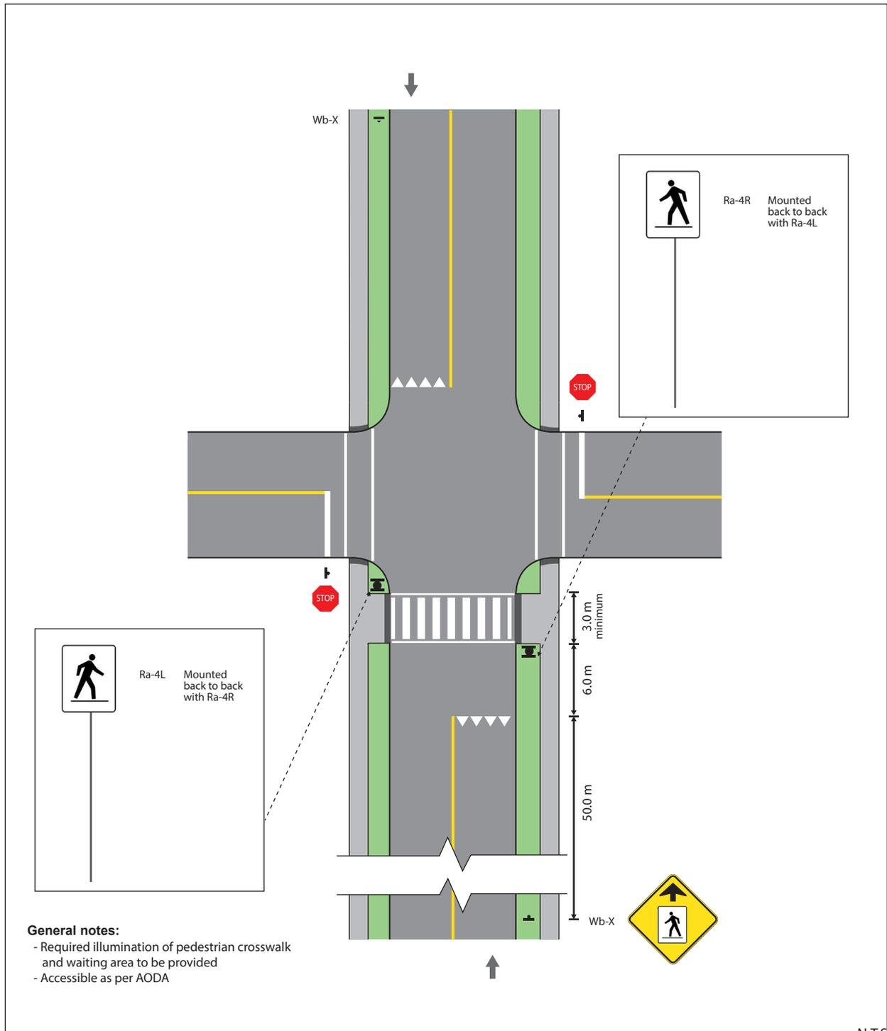
Figure 45: Pedestrian Crossover Type D – Intersection (2-way)
