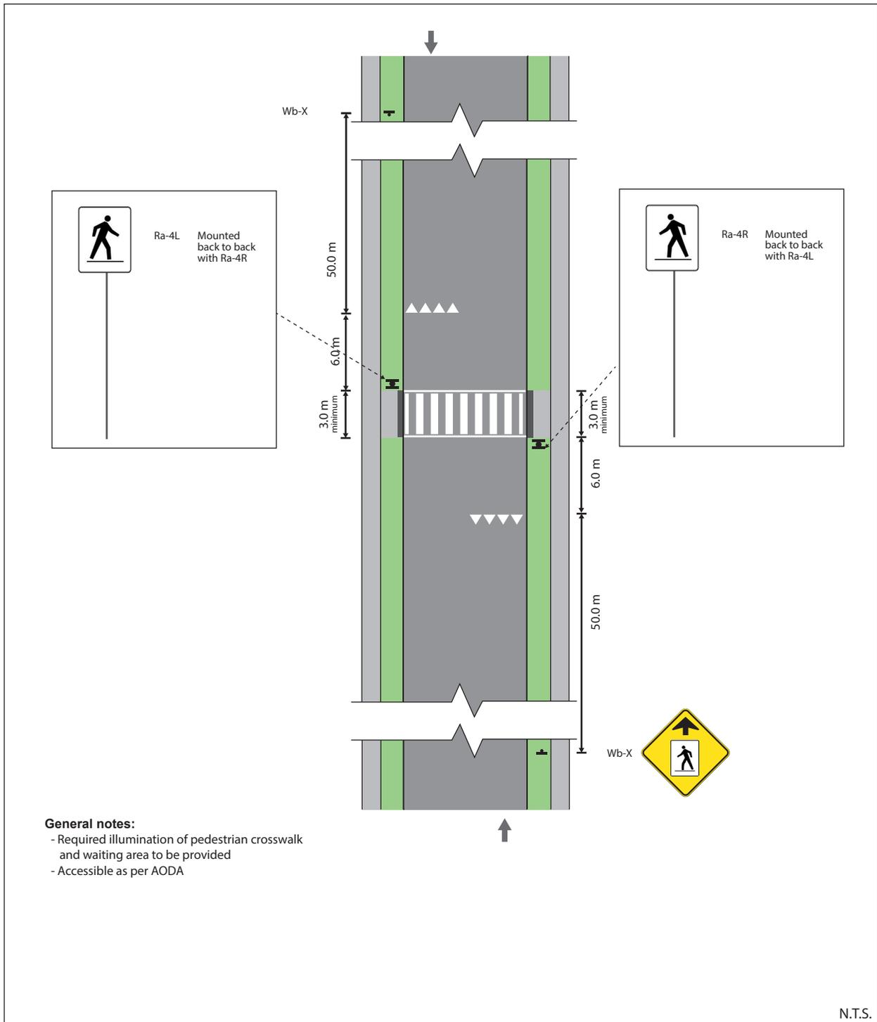
Figure 40: Pedestrian Crossover Type D – Mid-block (2-lane, 2-way)
