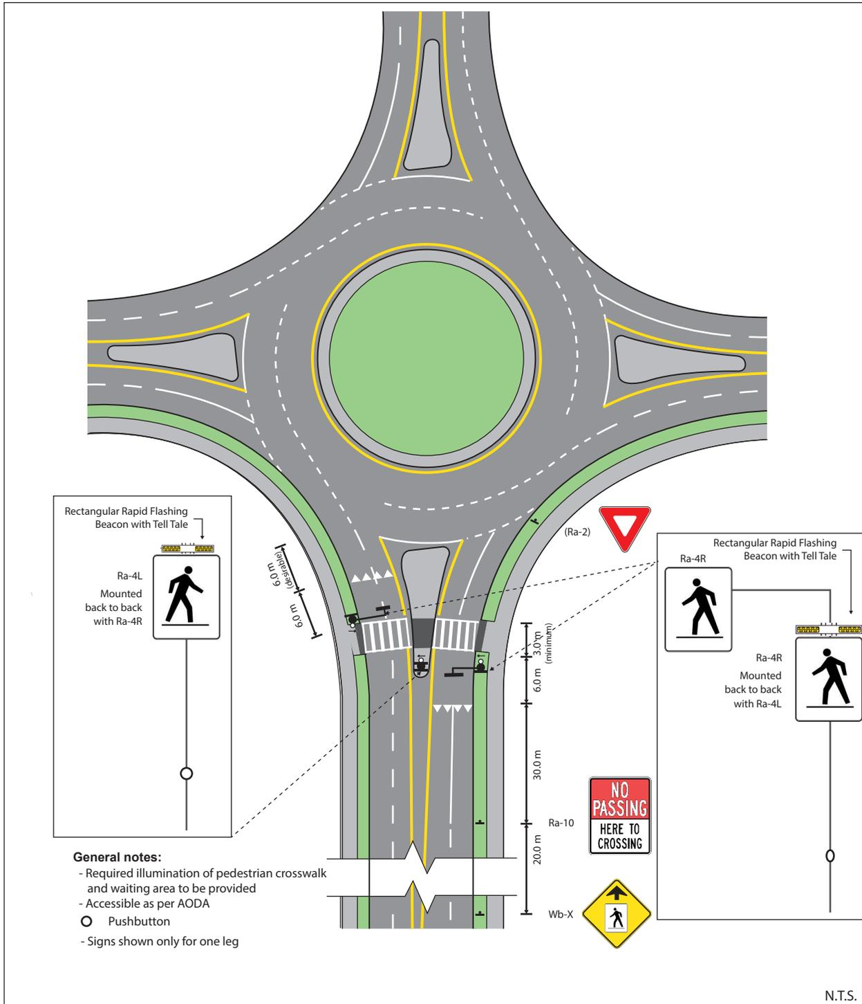
Figure 30: Pedestrian Crossover Type B – Double-Lane Roundabout
