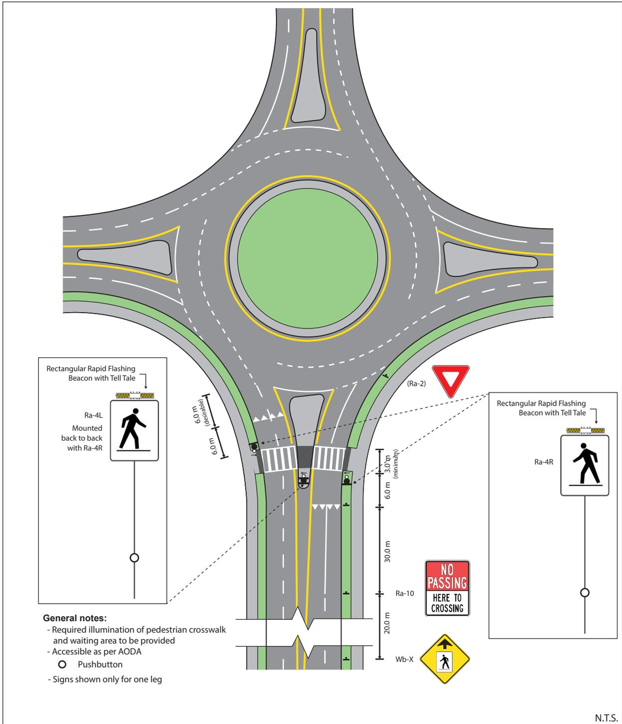
Figure 39: Pedestrian Crossover Type C – Double-Lane Roundabout
