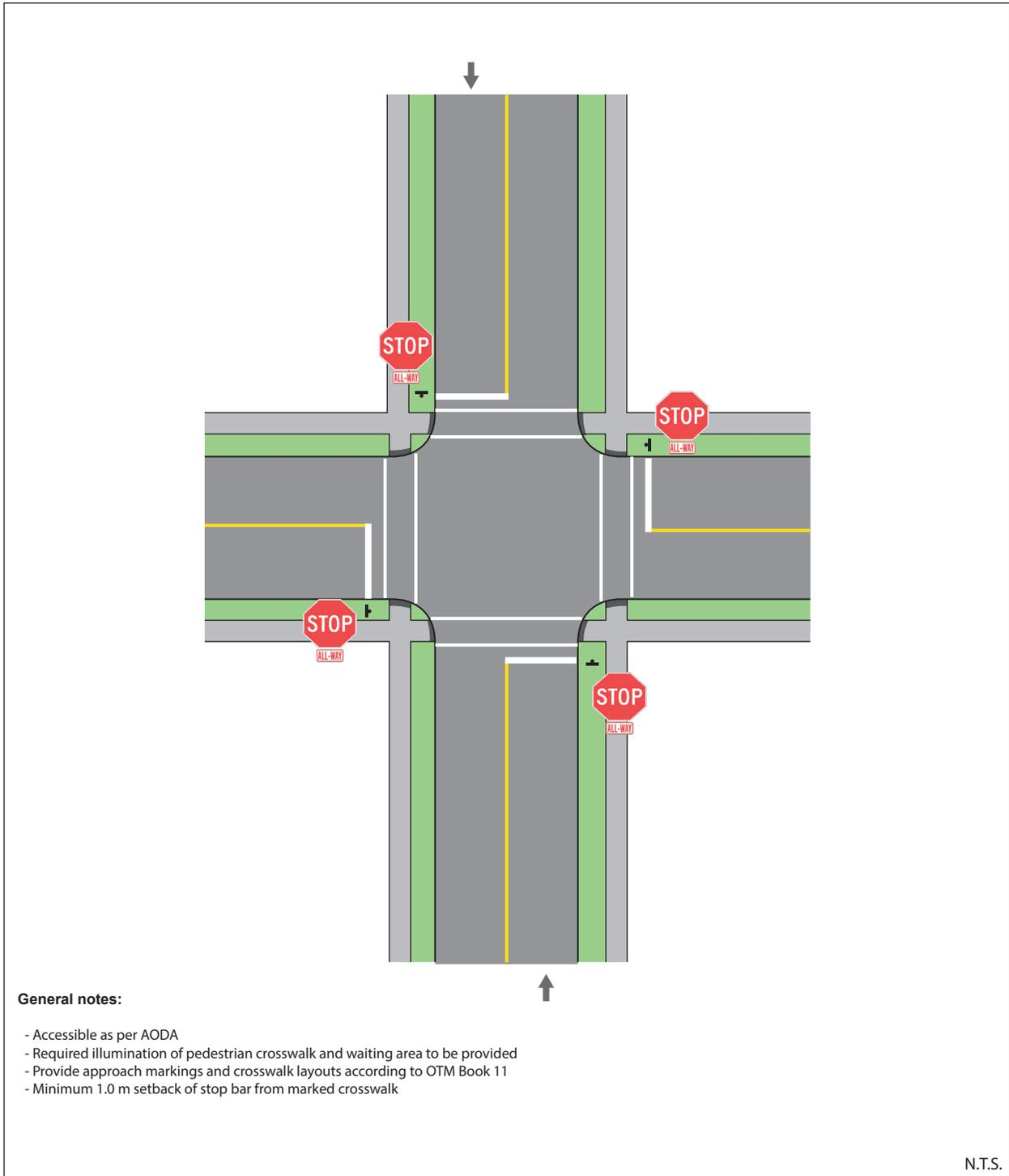
**Figure 49: Stop Controlled Intersections as Pedestrian Crossing Treatment**
