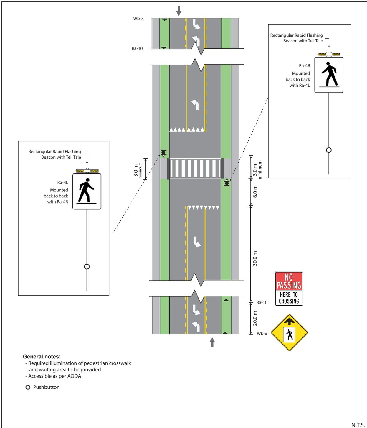
**Figure 32: Pedestrian Crossover Type C – Mid-block (3-lane with centre 2-way left-turn lane)**
