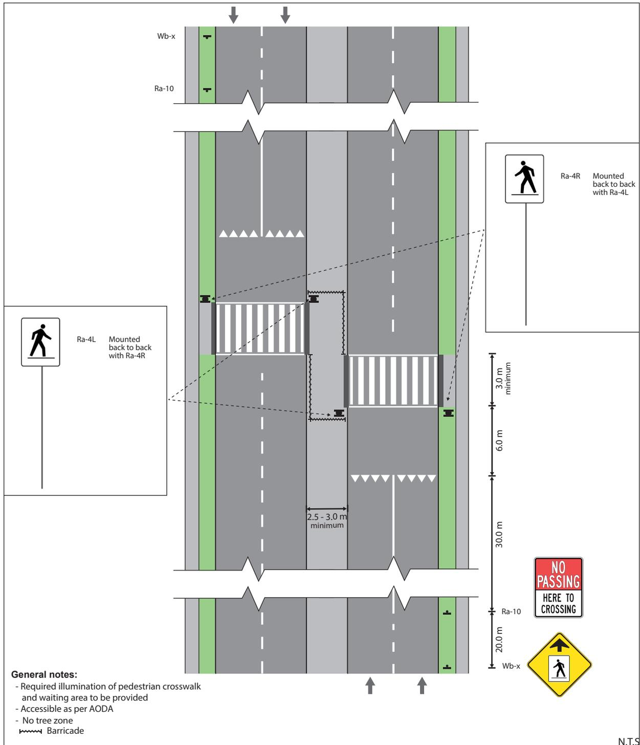
**Figure 41: Pedestrian Crossover Type D – Mid-block (4-lane, 2-way with raised refuge)**
