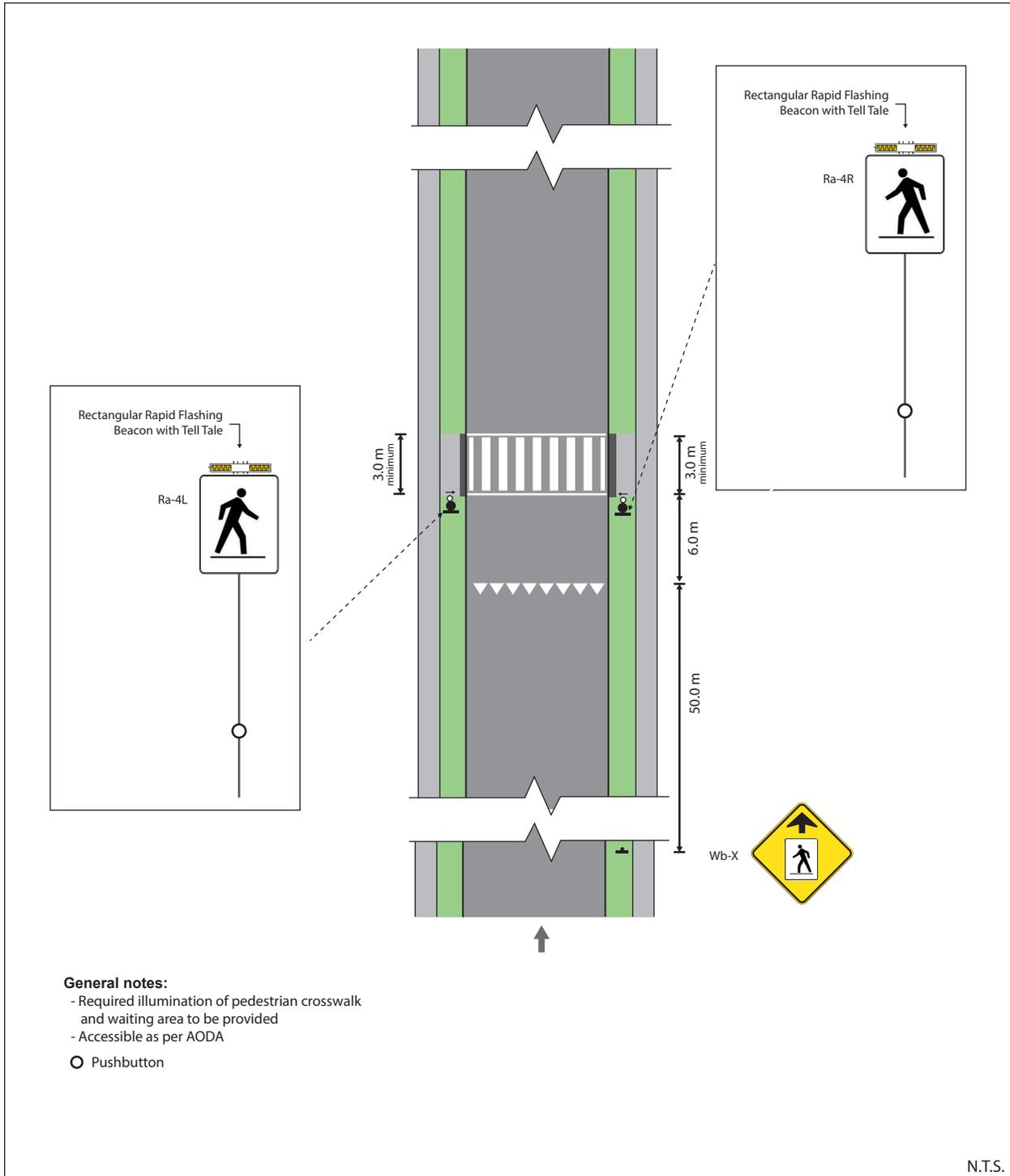
Figure 34: Pedestrian Crossover Type C – Mid-block (1-lane, 1-way)
