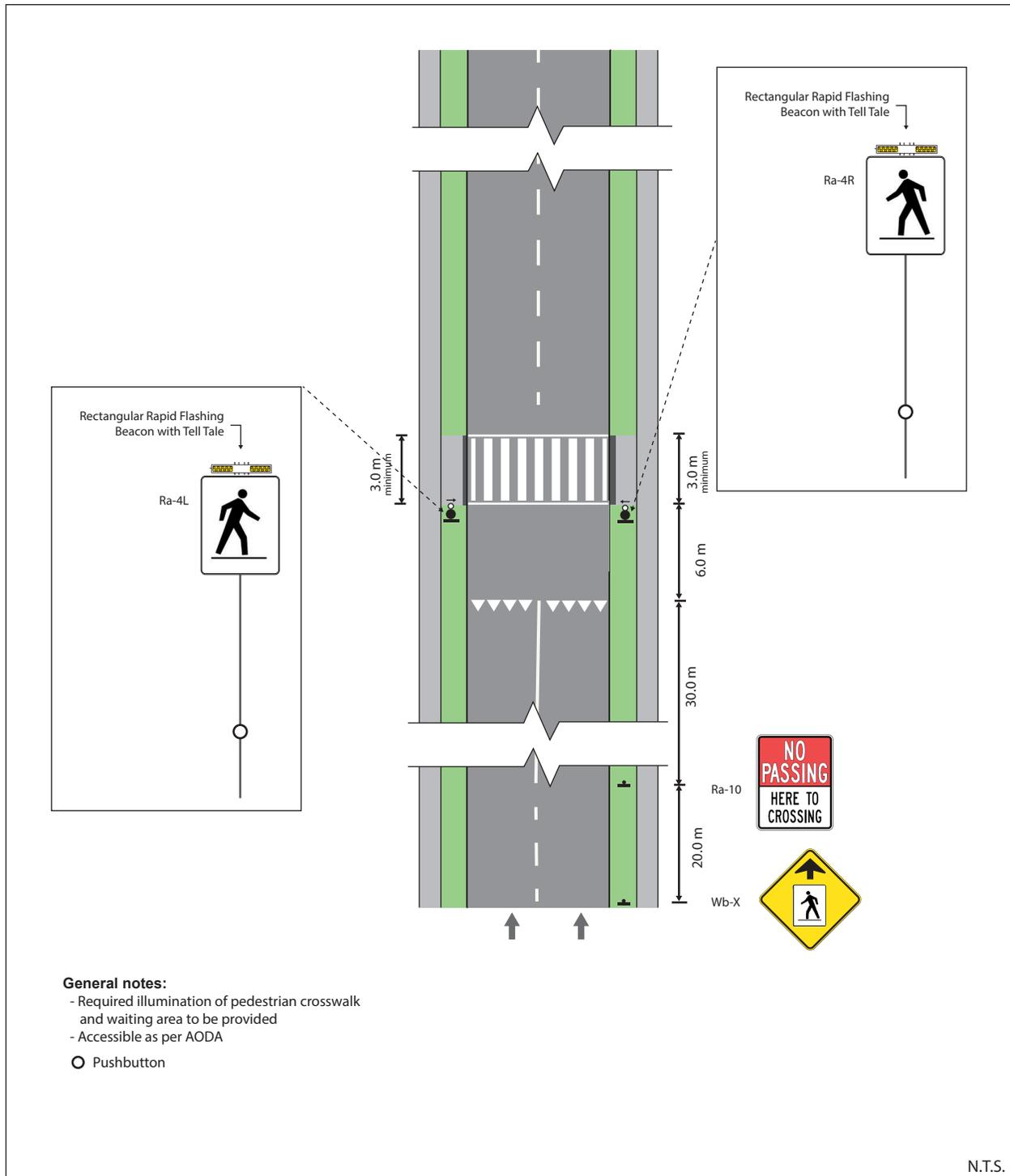
Figure 35: Pedestrian Crossover Type C – Mid-block (2-lane, 1-way)
