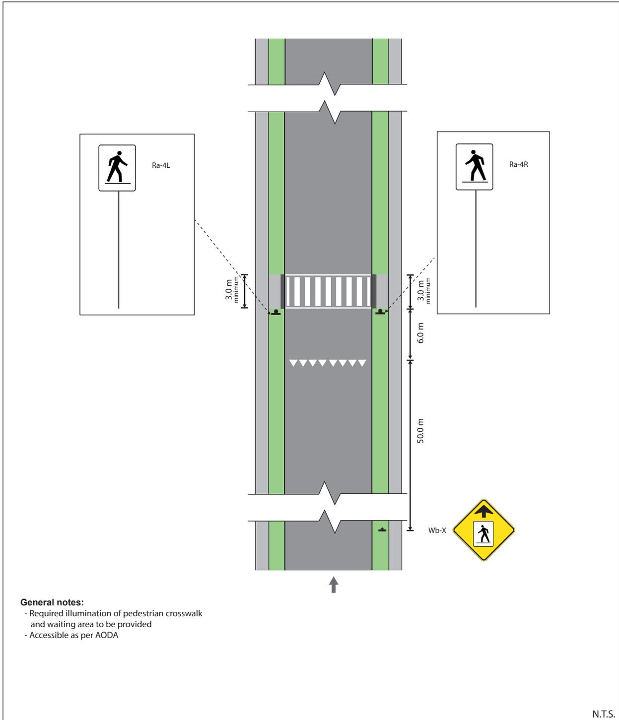
Figure 42: Pedestrian Crossover Type D – Mid-block (1-lane, 1-way)
