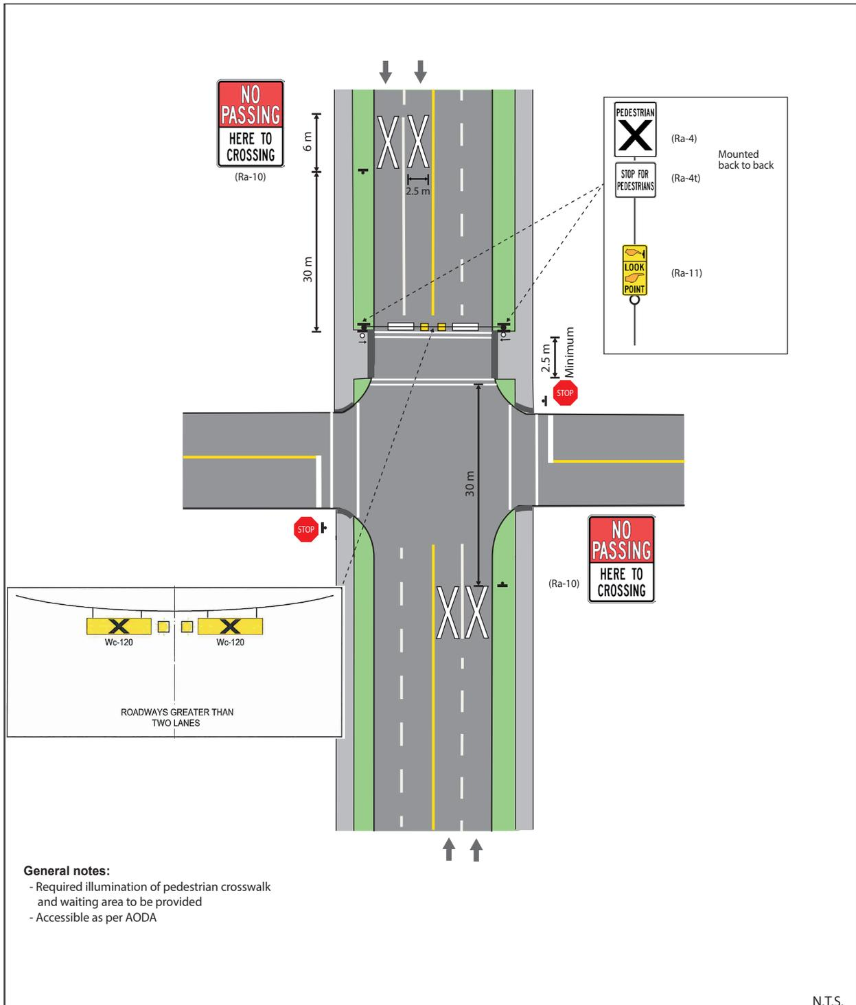
Figure 20: Pedestrian Crossover Type A – Intersection (2-way)
