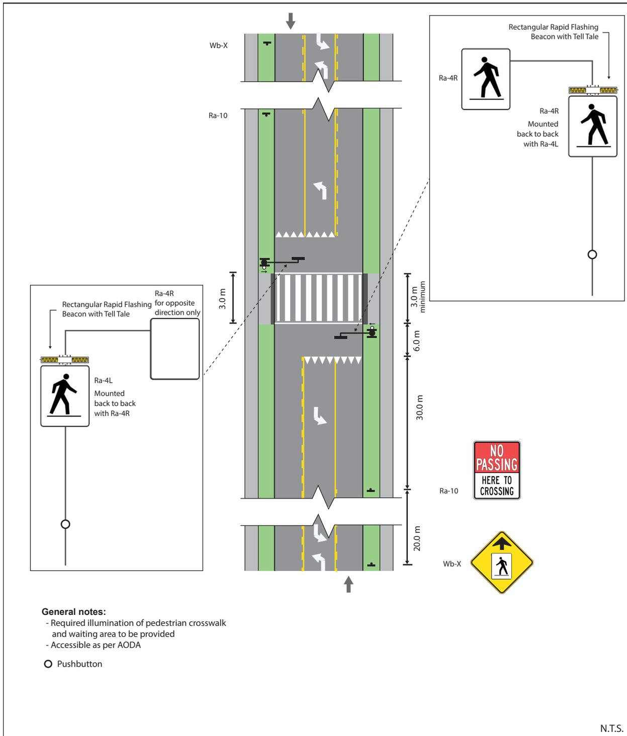
Figure 23: Pedestrian Crossover Type B – Mid-block (3-lane with centre 2-way left-turn lane)
